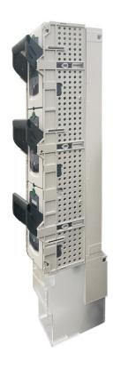
NH stands for "low voltage high rupturing capacity" (from the German: Niederspannungs Hochleistungs Sicherungen). NH fuses have a breaking capacity generally exceeding 100 kA, which covers virtually all the short-circuit currents expected to be encountered in low voltage systems.
