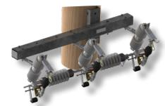
Electronic Sectionalisers have been developed for usage on overhead distribution lines to eliminate transient faults. They are typically used in conjunction with a recloser and replace the traditional dropout fuse protection.
